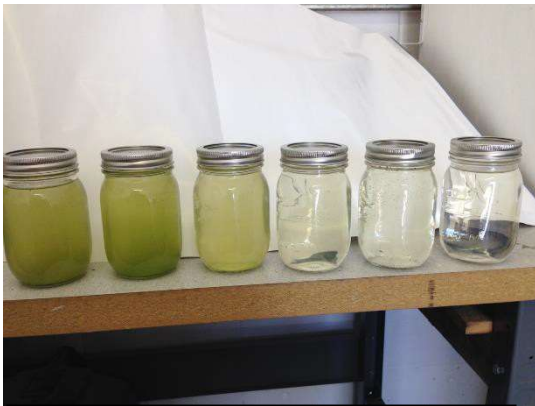
Figure 3. Effluent from Each Cell in the System and the Chlorine Contact Chamber
