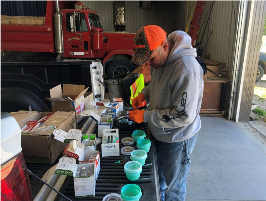
Figure 4. Scott Zortman with the Mahnomen Wastewater System Testing for Ammonia and Ortho-Phosphorous
