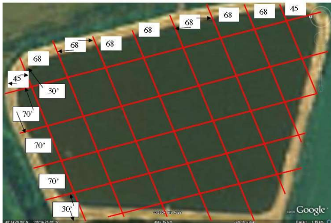
Figure 2. A Sludge Judging Grid Created from a Satellite Image
