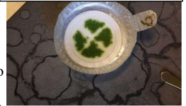
Figure 1. TSS Filter. Effluent TSS 105 mg/l Courtesy of Mark Court, Wyoming Rural Water
